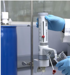
Remote Dispensing System for Drum Dispensing
